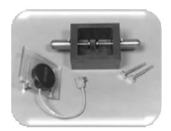
Test Cell: TCCE90 ASTM D877 ASTM D1816
